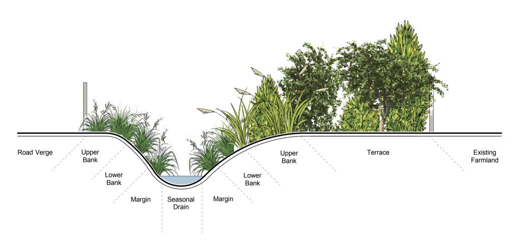
Note: Retain access on one side of drain for cleaning/maintenance purposes.
