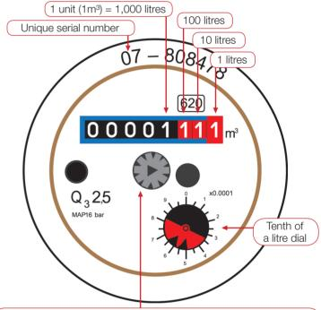
Spinner – spins rapidly when water is used – may move slowly if you have a small leak, a dripping tap or while a ball valve is closing
