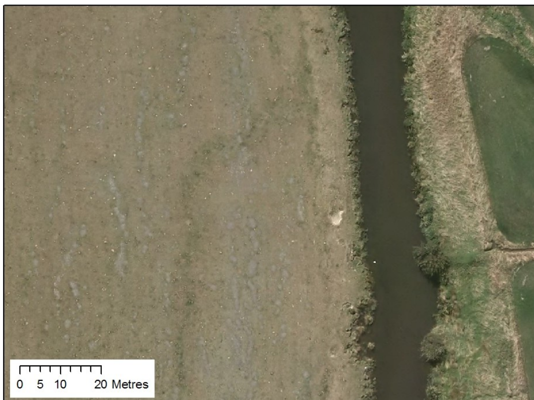
Figure A3.7 Liquefaction adjacent to the Styx River, west of Brooklands, February 2011. This area was also affected in September 2010 (image NZAM_mosaic_03_03_2011.ecw; centre of view approximately 1574970, 5194550).
