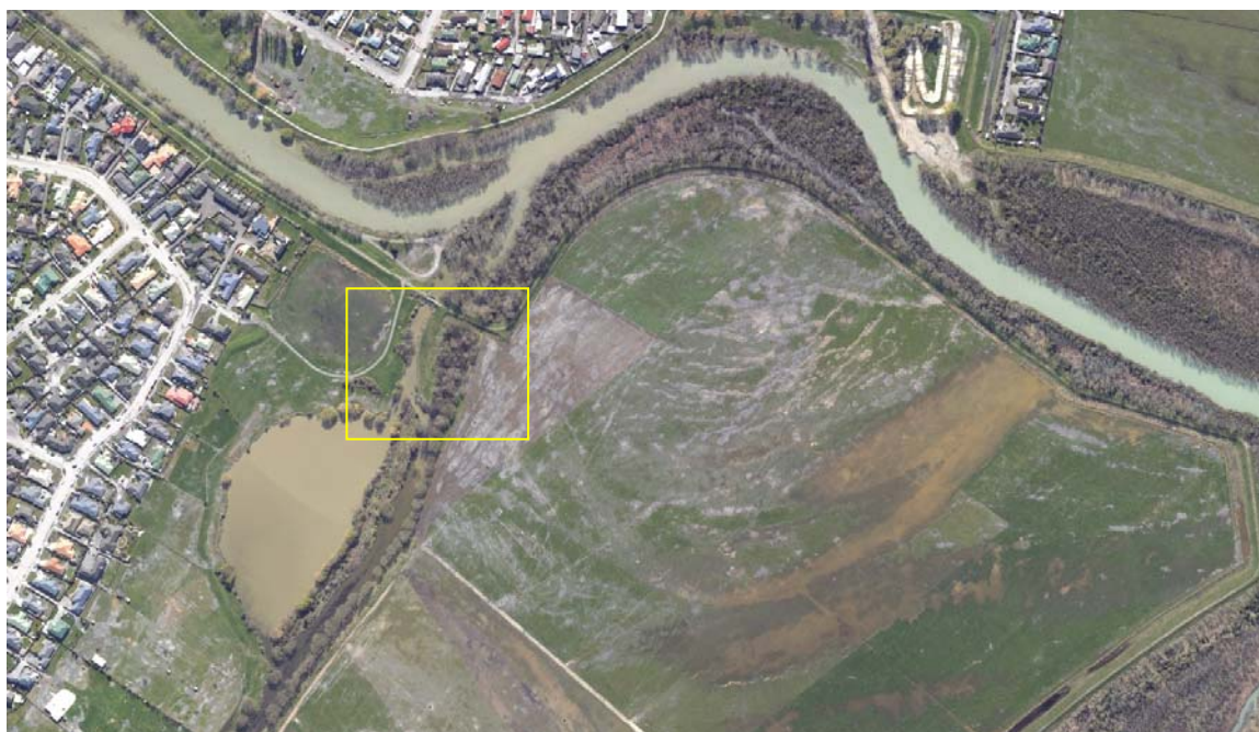
Figure A3.4.1 Liquefaction (sand boils, cracking/lateral spread and fissures) east of Kaiapoi, September 2010. Image is NZAM CANT_ortho_Kaiapoi; centre of view approximately 1573200, 5195800 (NZTM). Rectangle indicates location of detail shown in Figure A3.4.2.
