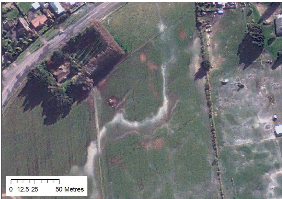
Figure A3.5 Liquefaction at Rawhiti, south of Halswell, September 2010. Damage includes cracking/lateral spread of the road, and sand boils and flooding (including sedimentation) in the paddocks (image Christchurch_GeoEye_4-9-10-All_data_Ortho.ecw; centre of view approximately 1564800, 5173000).
