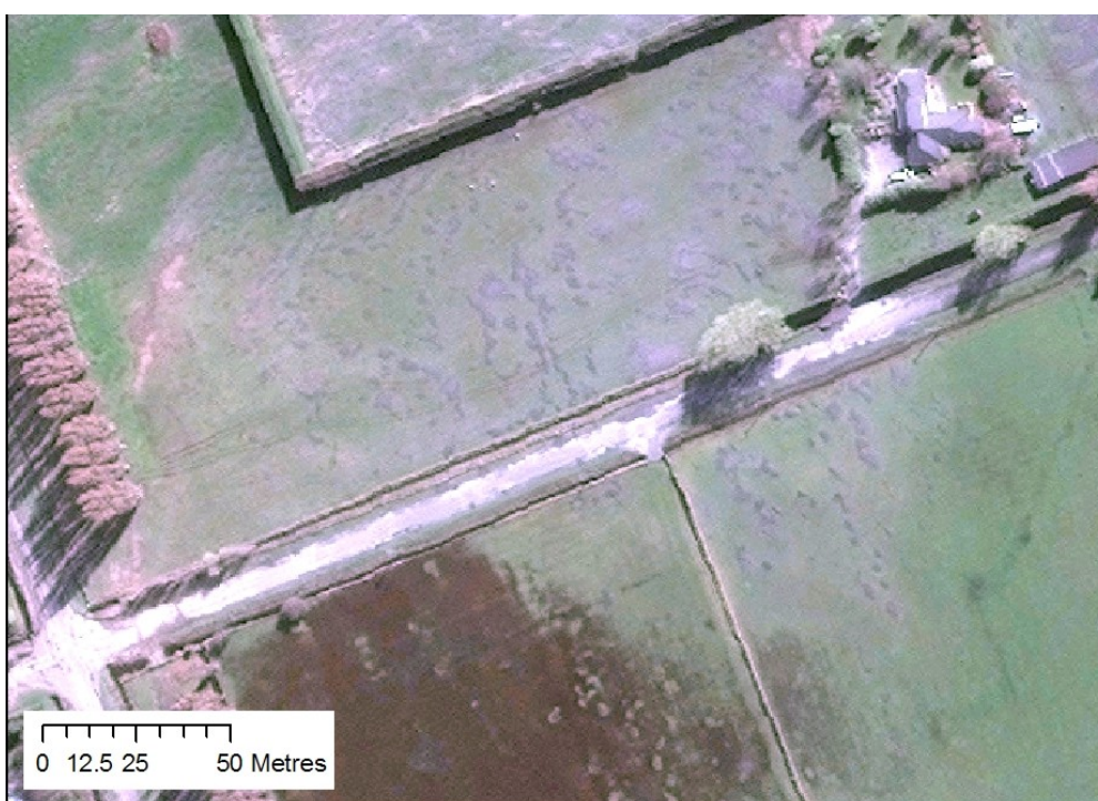
Figure A3.6 Sand boils and surface flooding across Carters Road, southwest of Tai Tapu, September 2010 (image Selwyn_DG_12_Sept_2010.img; centre of view approximately 1560000, 5164000).
