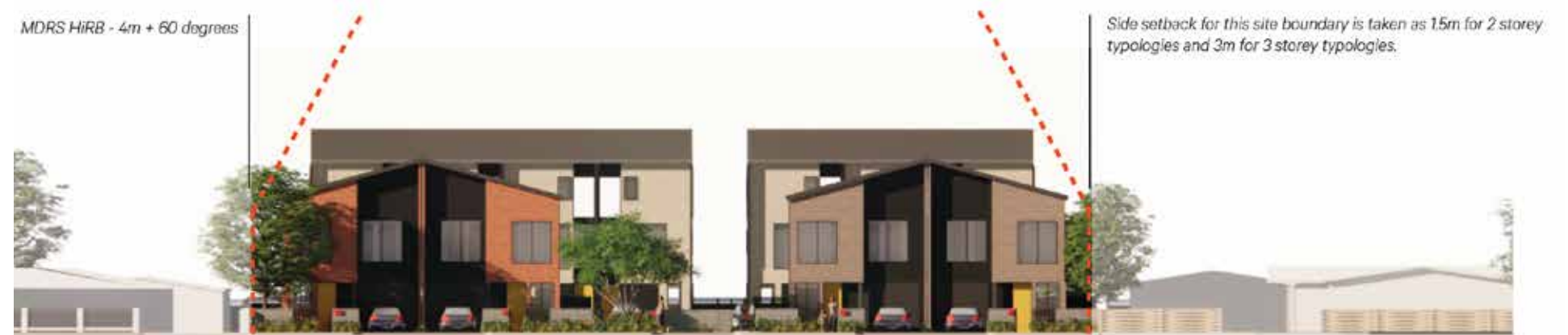
Image: Illustration of recession planes under the MDRS.
