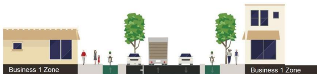
Figure 3.4 Cross section for Core Retail (East)
