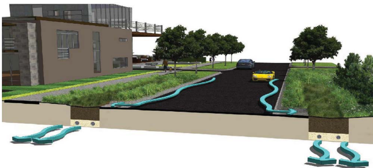
Figure 8.2: Capturing street runoff 'at-surface'
