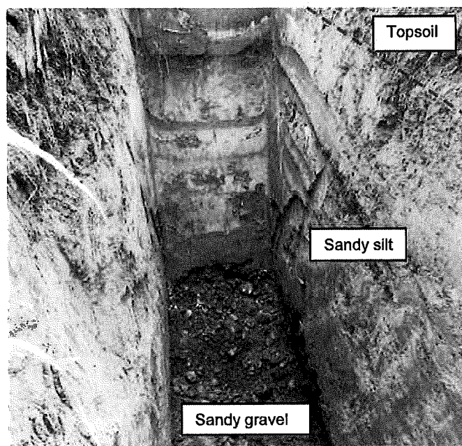
Photo 1: Sandy silt underlain by sandy gravel with cobbles and boulders to 2.0 m depth (TP3)
