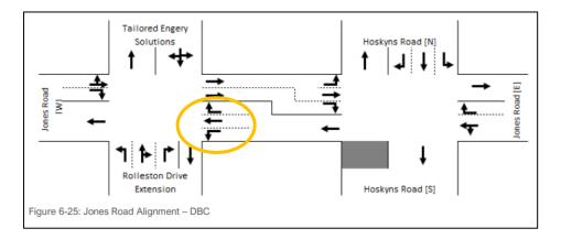
The alignment has now been changed with the straight and right turning traffic in one lane, and the other lane a left turning lane onto the overbridge, as shown below:
