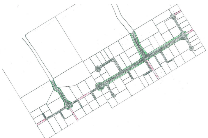
2—Cul-de-sac layout. Jozecom Place is extended. New cul-de-sacs are provided along the path of existing rights of way from Fairhurst Place. Jozecom and Fairhurst Places are connected by footpaths (shown in red).
