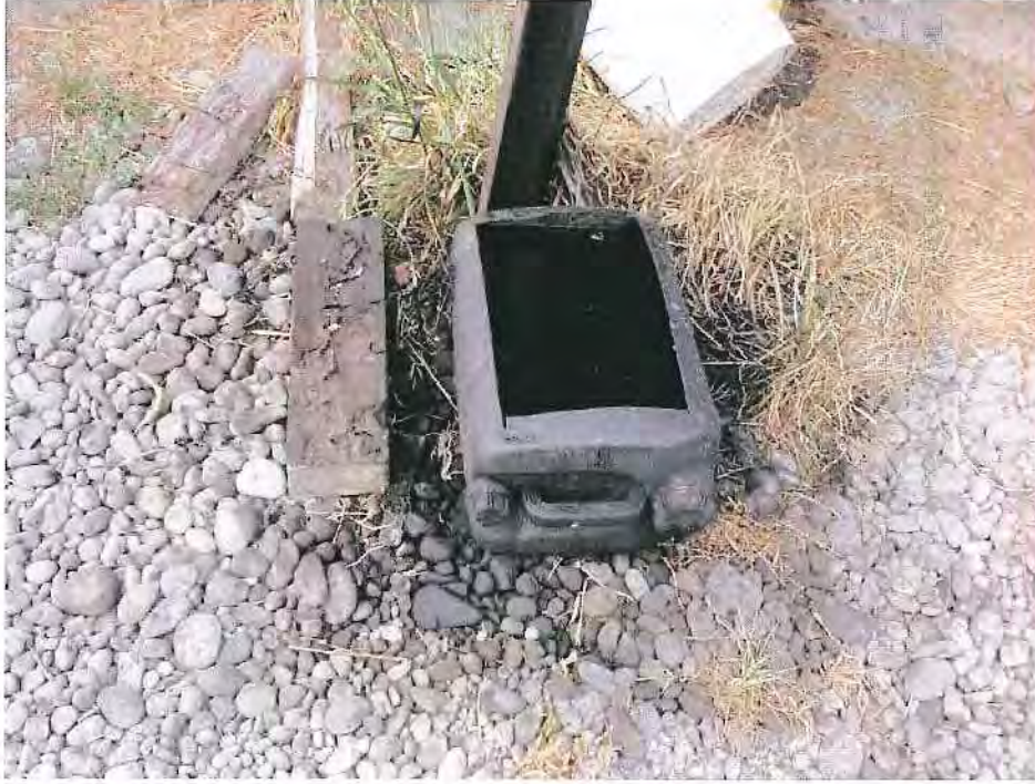
Photograph 10 : Container Filled With Waste Oil – Note Staining of Surrounding Ground
