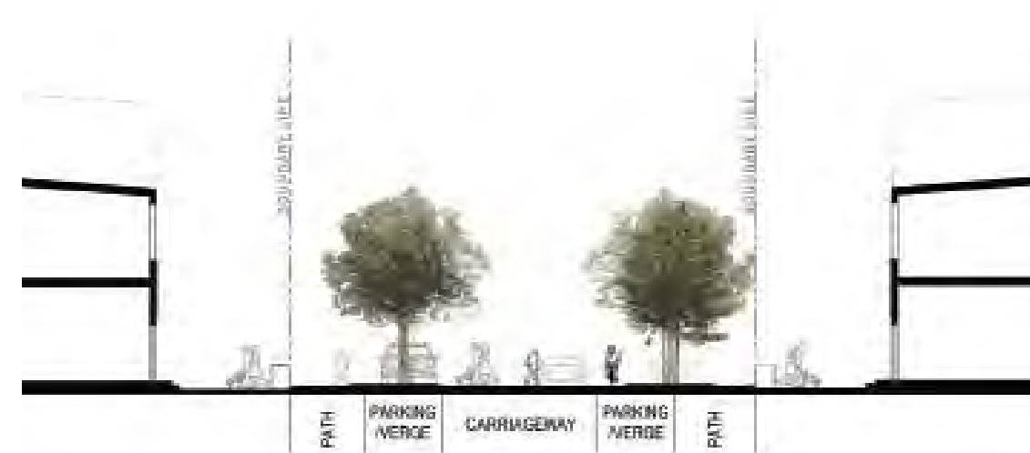
Figure 36: Section AA – Indicative section through compact residential street
