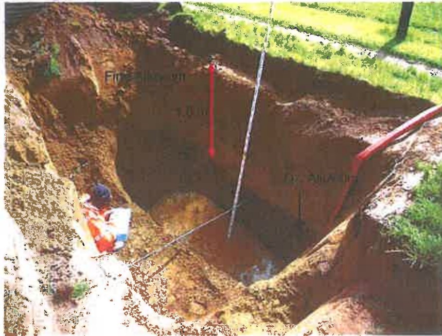
Figure 3. Photograph of Infiltration test of gravelly Q1a Alluvium in inspection pit TP3
