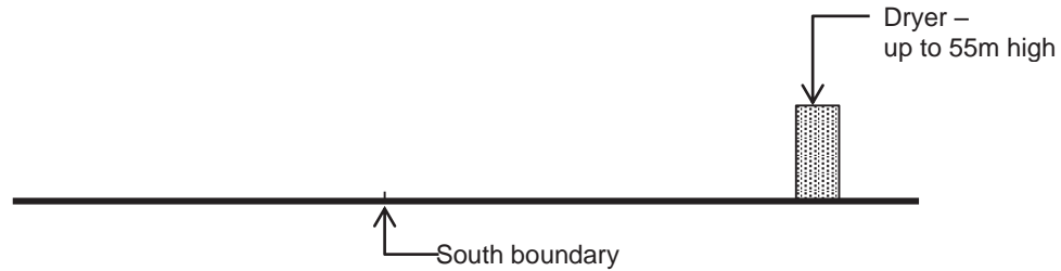
Figure 2 Showing the recession plane off the southern boundary closest to the potentially tallest buildings – the dryers. This demonstrates that there is no prospect that the dryers will shade neighbouring properties beyond what is anticipated by the District Plan.
