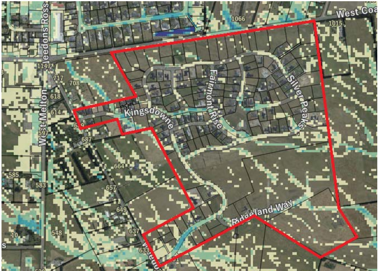
Figure 7 – Modelled flood extent, 0.5% AEP event, incorporating 8.5 RCP climate change scenario.
