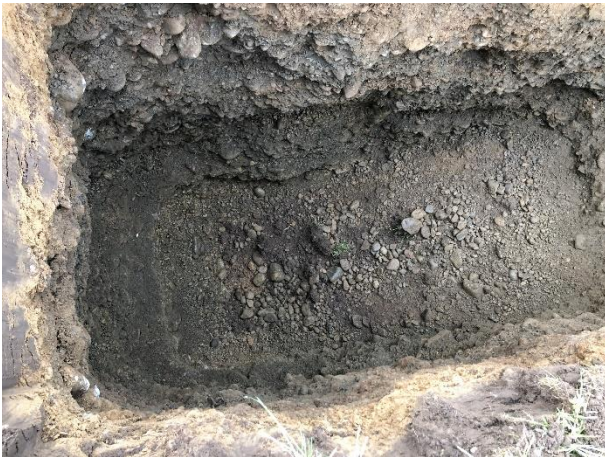
Photo 3. Small test pit (TP3) dug along western portion of the site. No fill noted- only natural silt.
