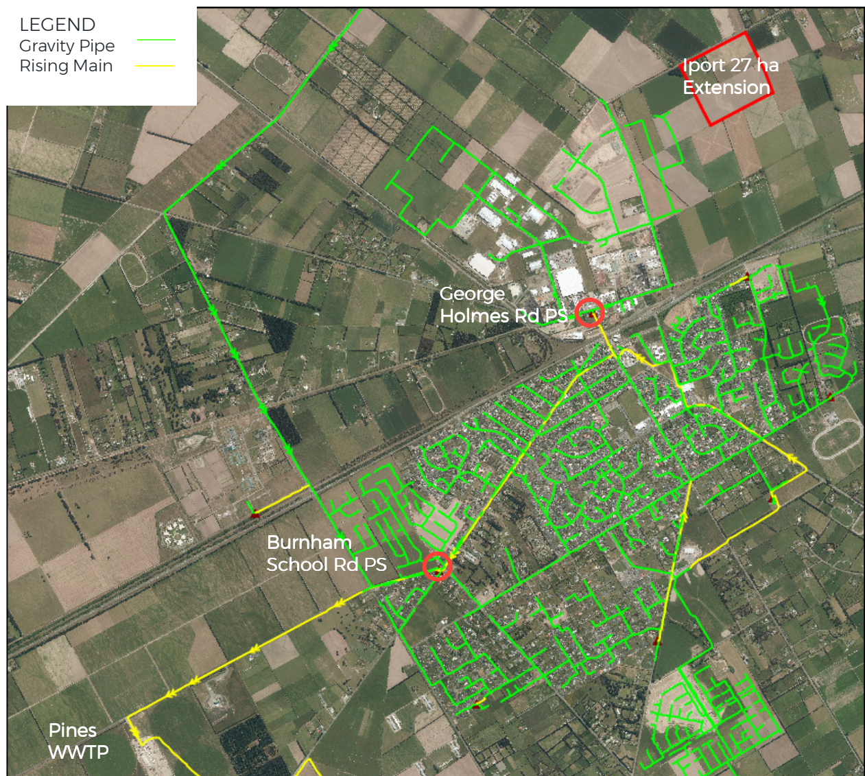
Figure 1 Wastewater System Overview
