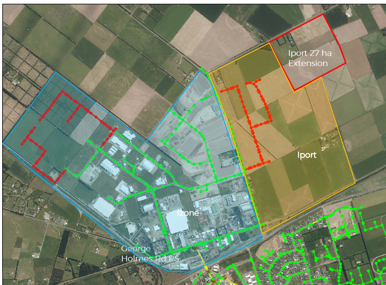
Figure 2 Wastewater model updates (added pipework shown in red)
