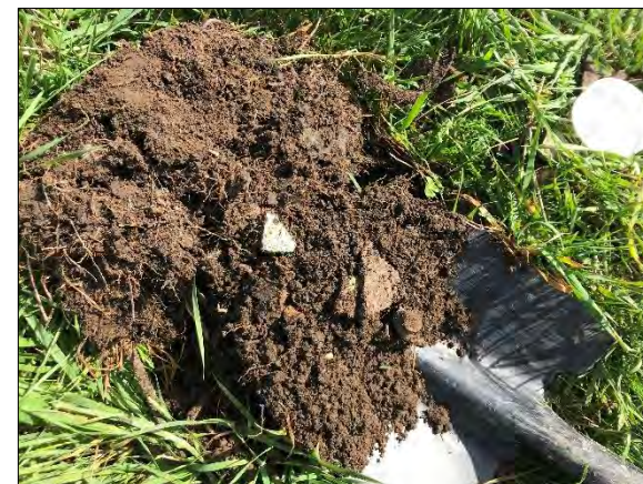
Photo 12: Asbestos cement board in burn pile material
