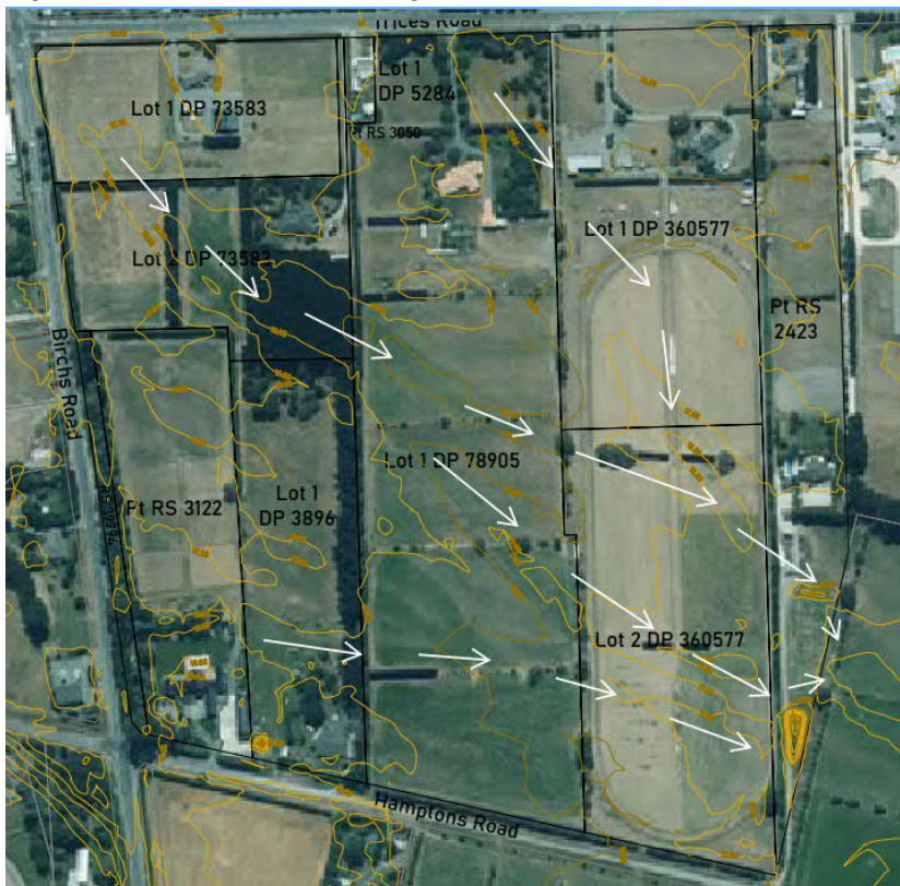
Figure 1 – Lidar & Local Drainage Routes
