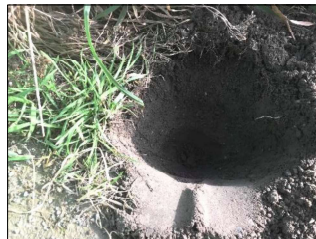
Photo 17: Typical soil profile below trotting track
