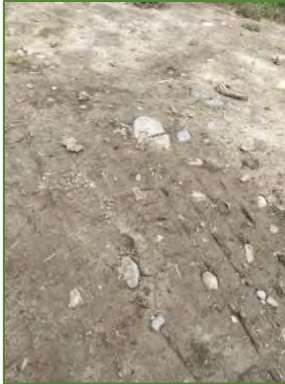
Photo 15 – Potential ACM fragments in vehicle track
