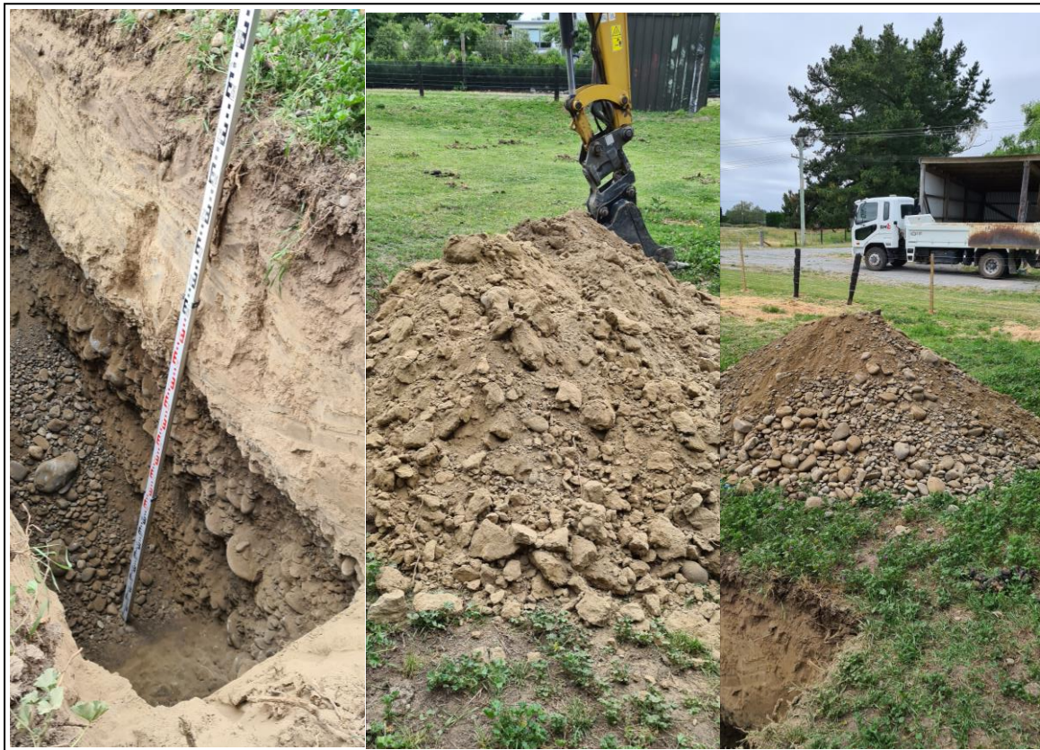
Photos 1: from left to right (1) Shows typical Test Pit excavation (2.6m deep), with loess and topsoil capping. (2) shows blocky excavated loess soils. (3) shows excavated river gravels.
