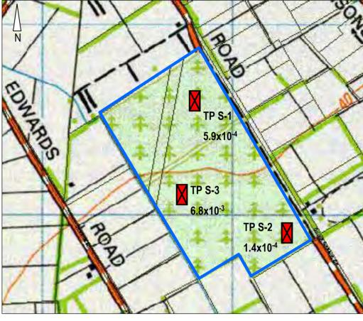
Approximate location of test pits with soak tests
