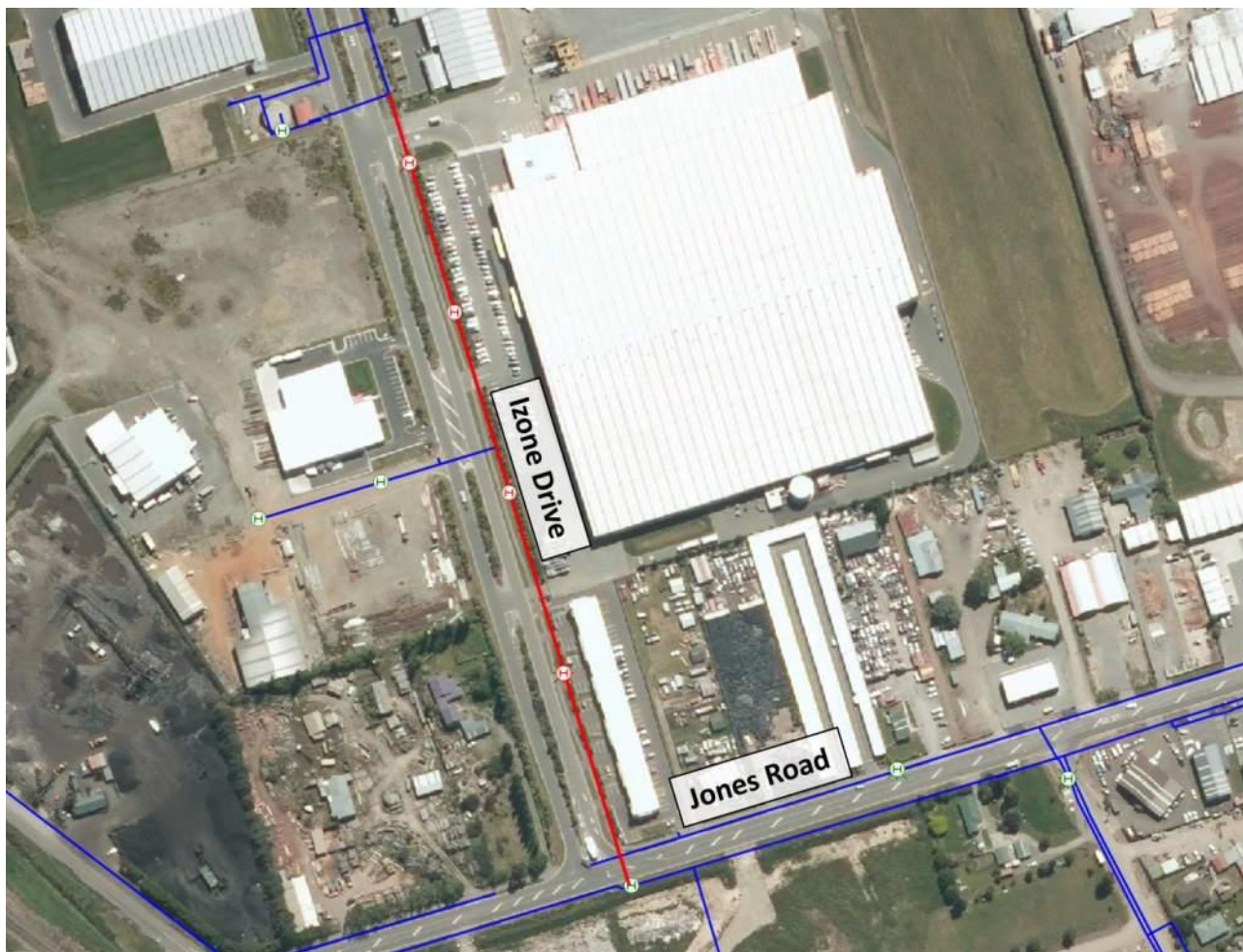
Figure 4-5: Pipe Upgrades Required to Service Two Chain Block (Upgrades Shown in Red)
