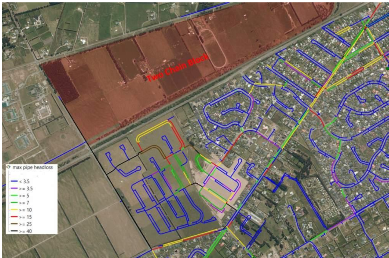
Figure 4-3: Option 2 Headlosses (m/km) in Rolleston Water Supply network
