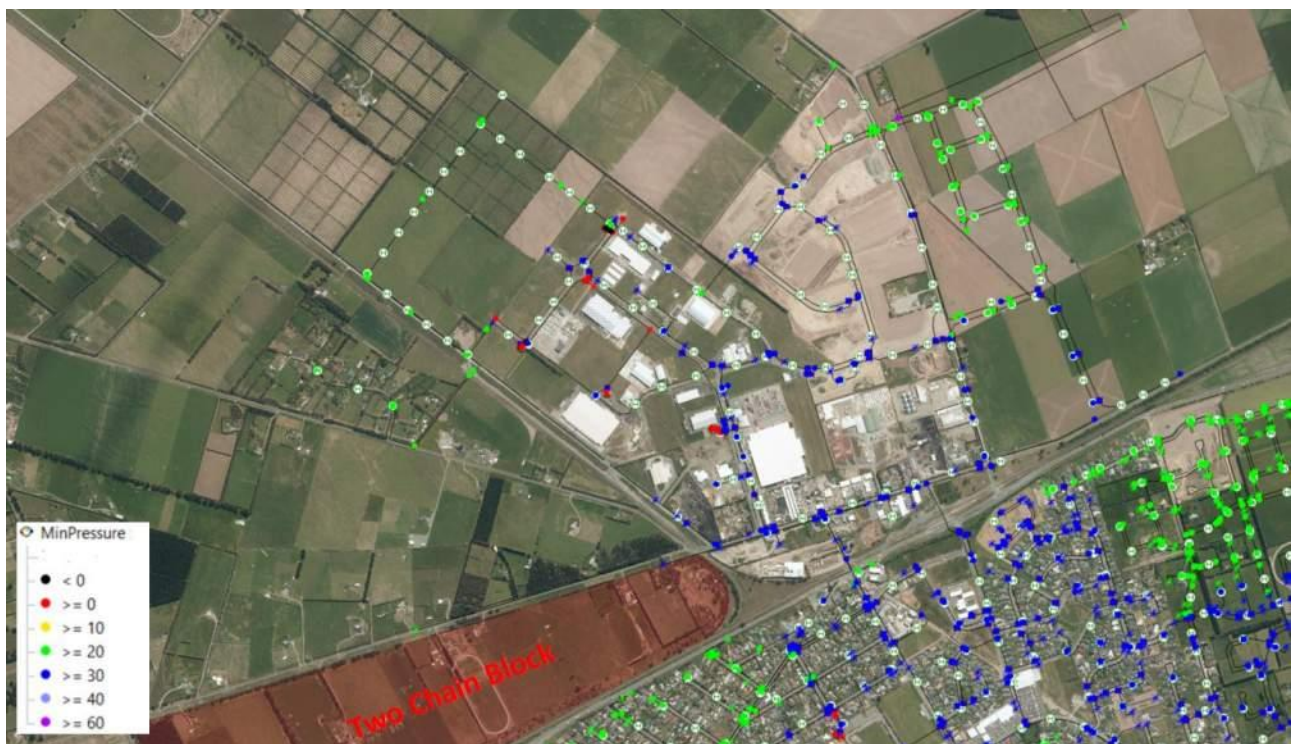
Figure 4-2: Option 1 Minimum pressure (m) in Rolleston Water Supply network
