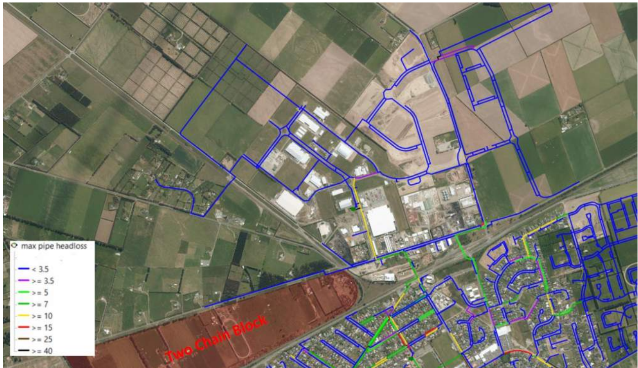
Figure 4-1: Option 1 Headlosses (m/km) in Rolleston Water Supply network
