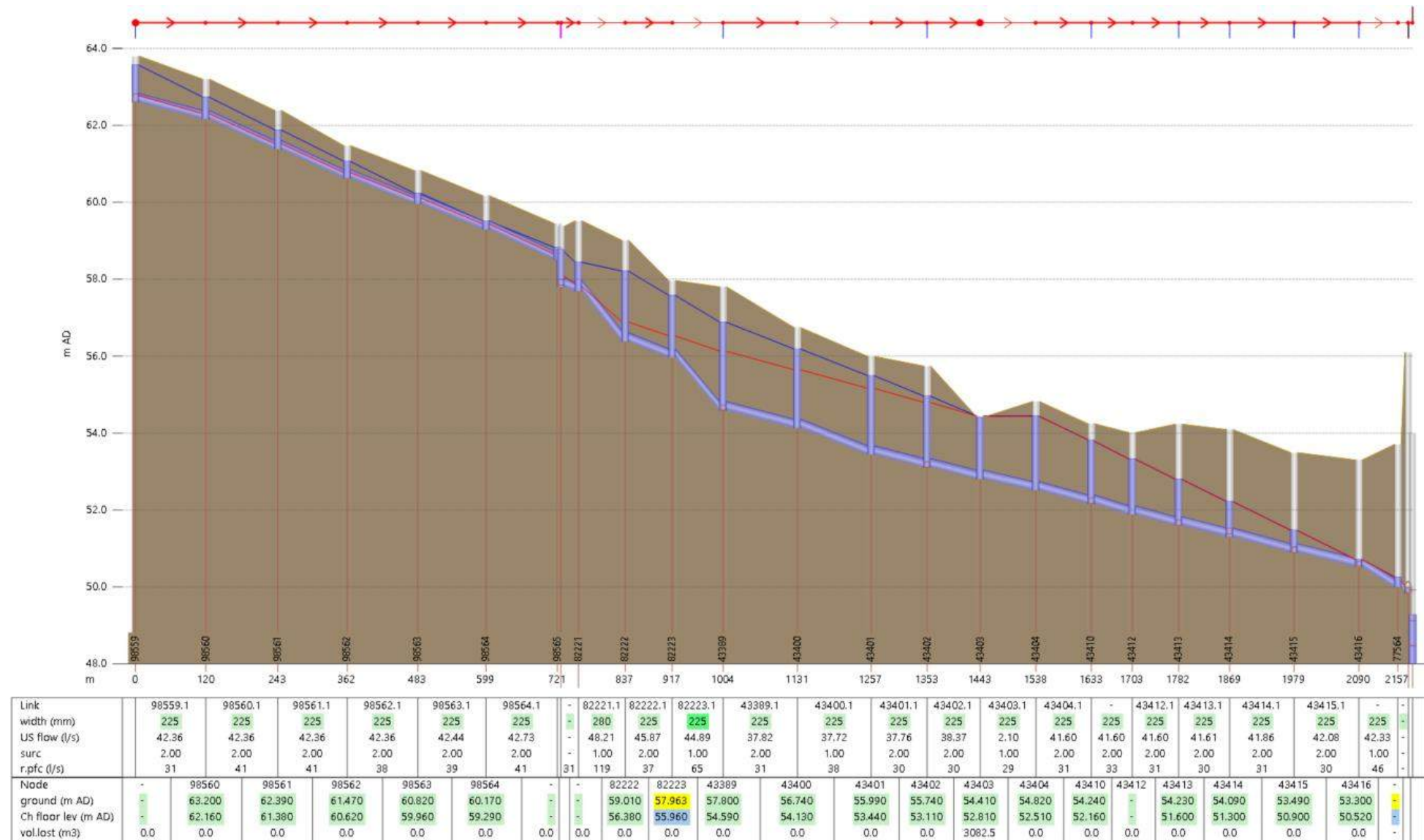
Figure 5-3: Long section at PWWF in the from manhole Asset ID 98559 to Burnham School Road PS. Predicted levels in the current system without the Two Chain Block is shown by the red line.
