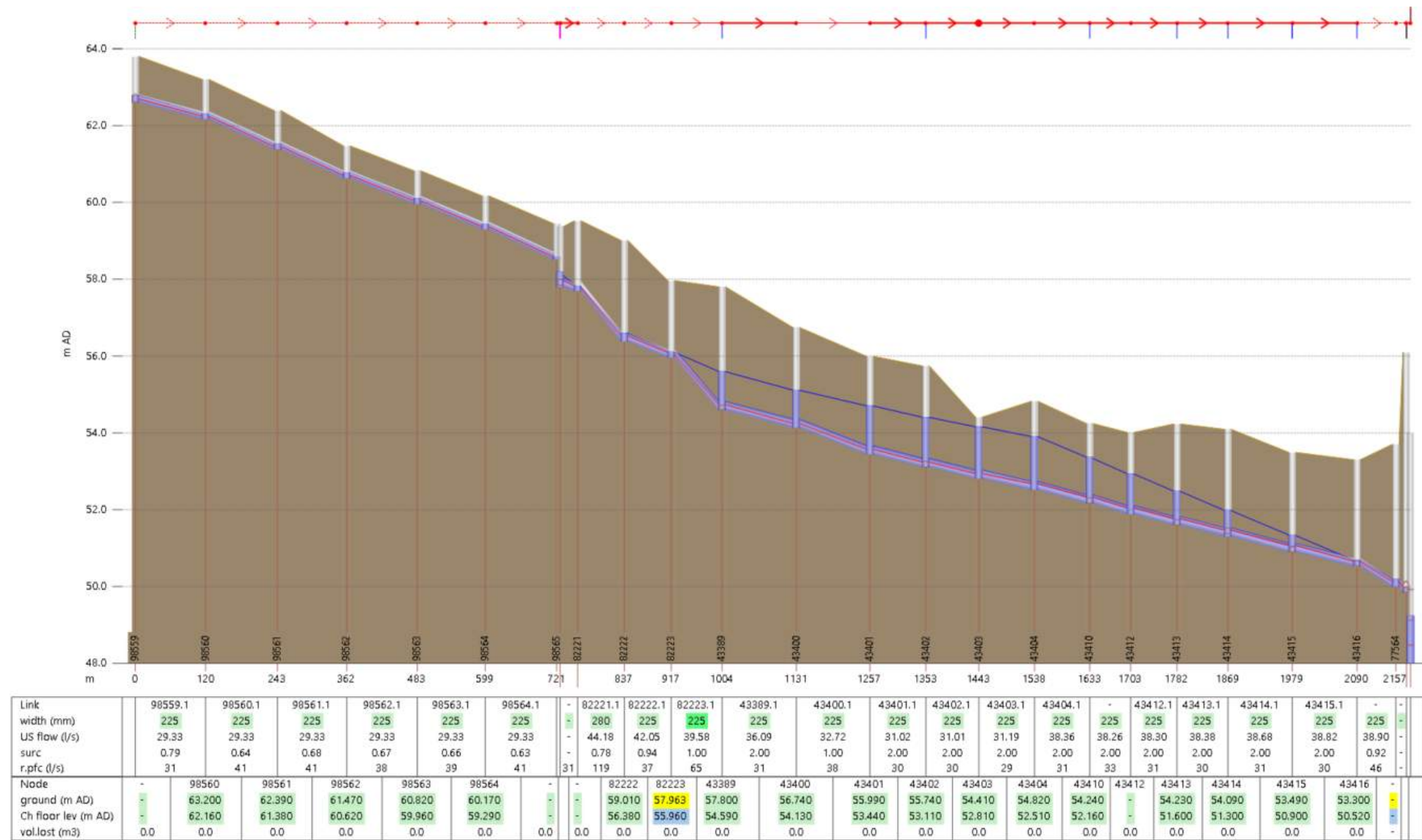
Figure 5-2: Long section at PDWF in the from manhole Asset ID 98559 to Burnham School Road PS. Predicted levels in the current system without the Two Chain Block is shown by the red line.
