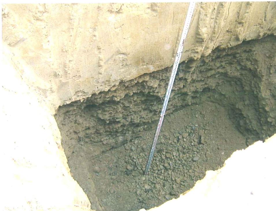
PHOTO: 2 NARRATIVE: Test pit 4. Note: Top layer sandy silt, bottom layer sandy gravel
