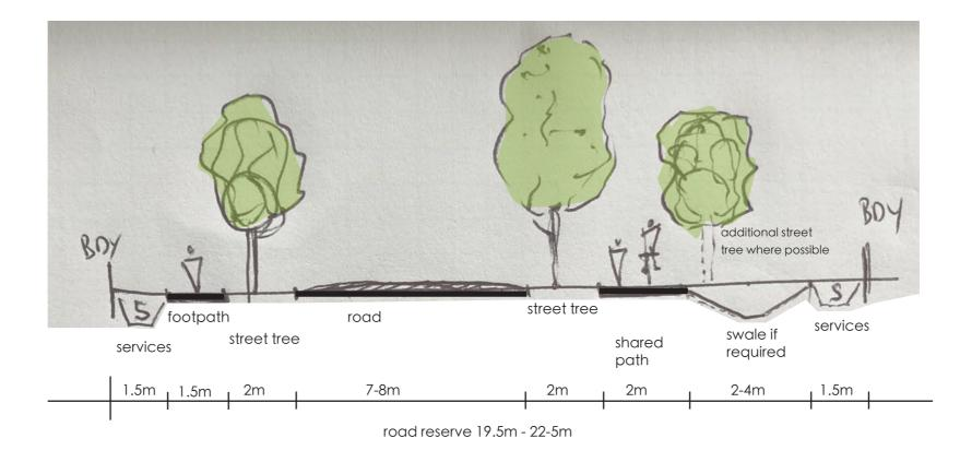
key primary roads with shared pedestrian and cycle way separated from main carriageway and stormwater conveyance
