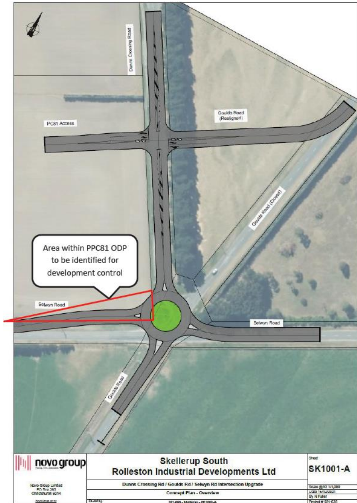
Figure 1: Concept design for the realignment of the Dunns Crossing Road/Selwyn Road/Goulds Road intersection
