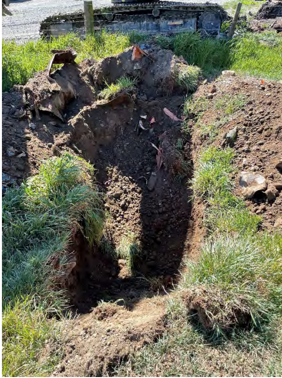
P37: Geotechnical test pit TP13 showing man-made materials (metal, glass bottles)
