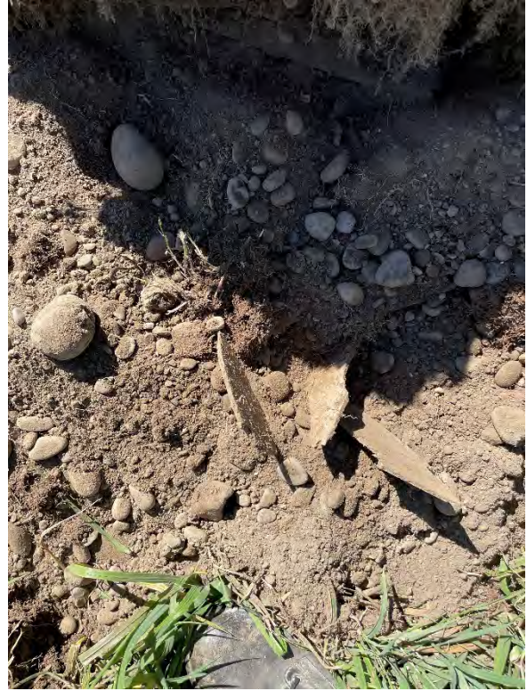
P38: Suspected ACM excavated from TP13
