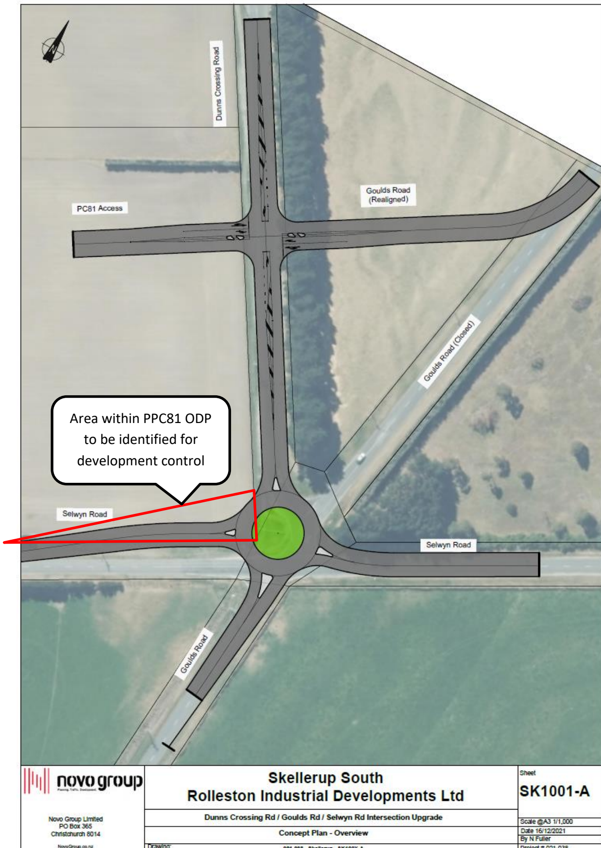
Figure 9: Concept plan for Dunns Crossing Road / Selwyn Road / Goulds Road intersection realignment and upgrade, and area that should be identified in the ODP for development control
