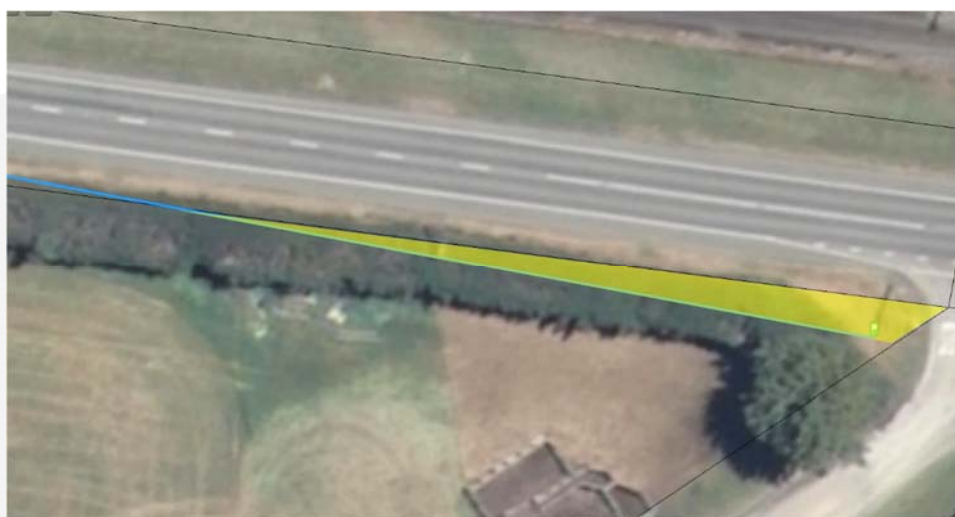
Figure 7: Land Potentially Required for Sightline towards West of (Realigned) Intersection (in Yellow)
