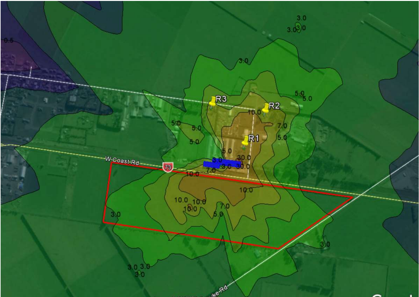
FIGURE 5 PREDICTED PM 10 24 HOUR AVERAGE CONCENTRATIONS (µg/M 3 ): COAL BURNING
