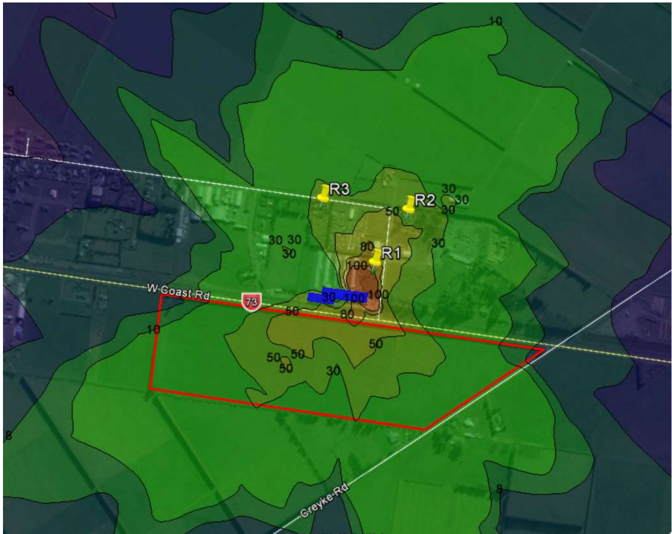
FIGURE 6 PREDICTED PEAK SO 2 24 HOUR AVERAGE CONCENTRATIONS (µG/M 3 ): COAL BURNING
