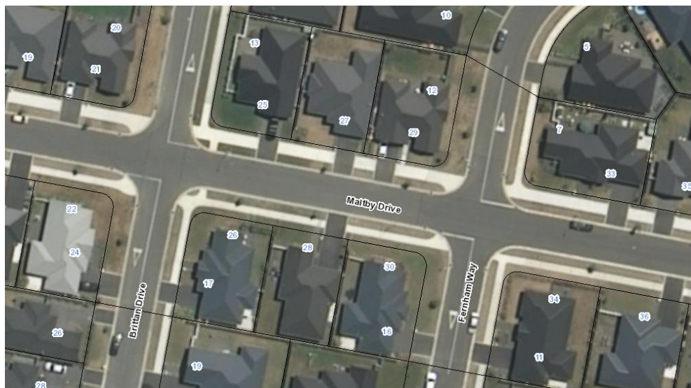
Figure 6.1 3m radius corner splays in a living zone (Faringdon)
