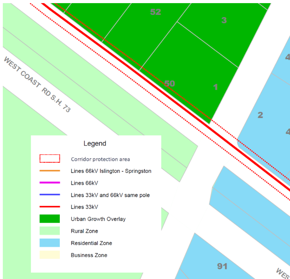
Figure 6: Example of electricity distribution corridor associated with 33kV line affecting slither of land within an urban growth overlay and existing residentially zoned land.
