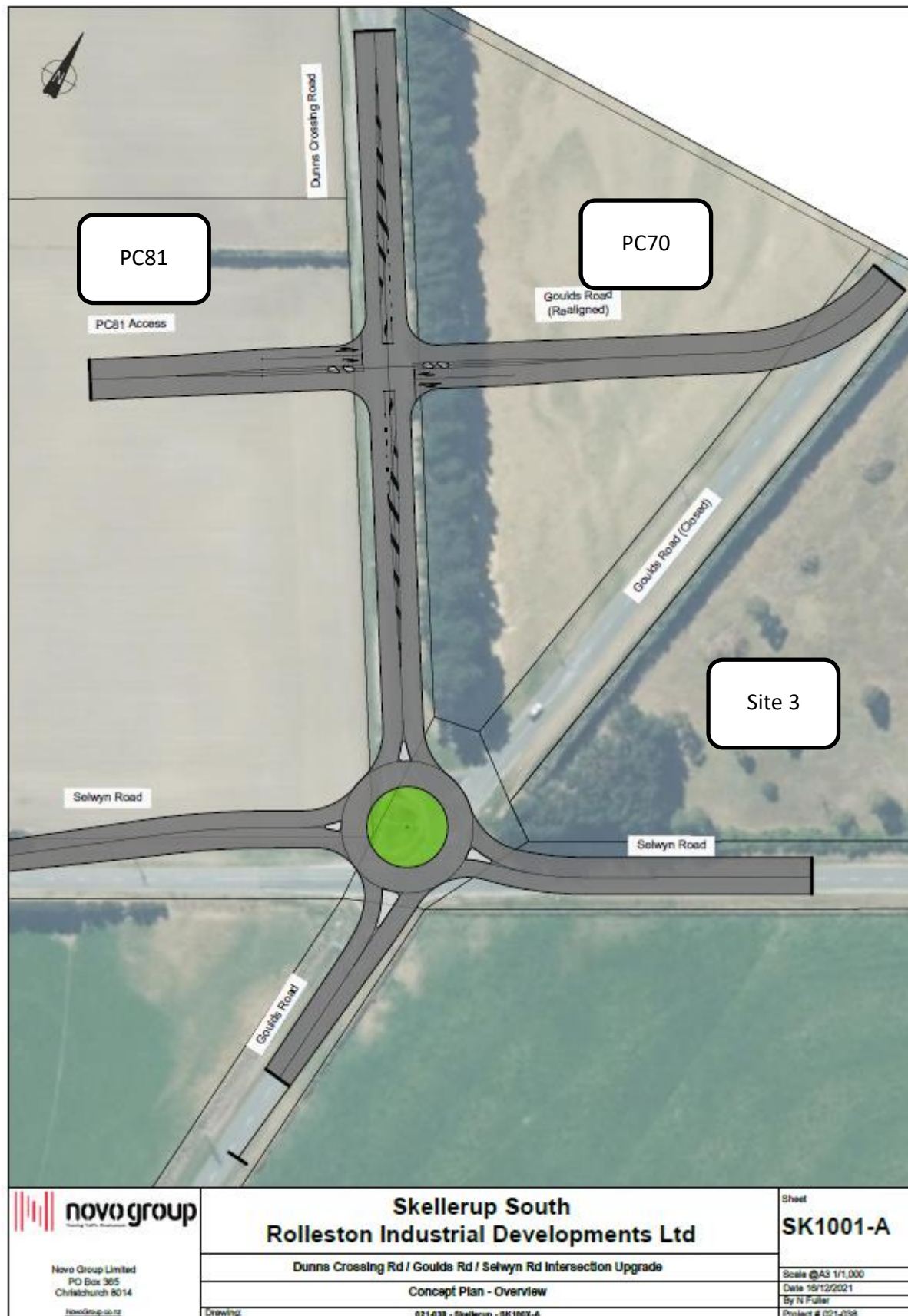
Figure 11: Indicative design for the upgrade of the Selwyn Road / Dunns Crossing Road / Goulds Road intersection
