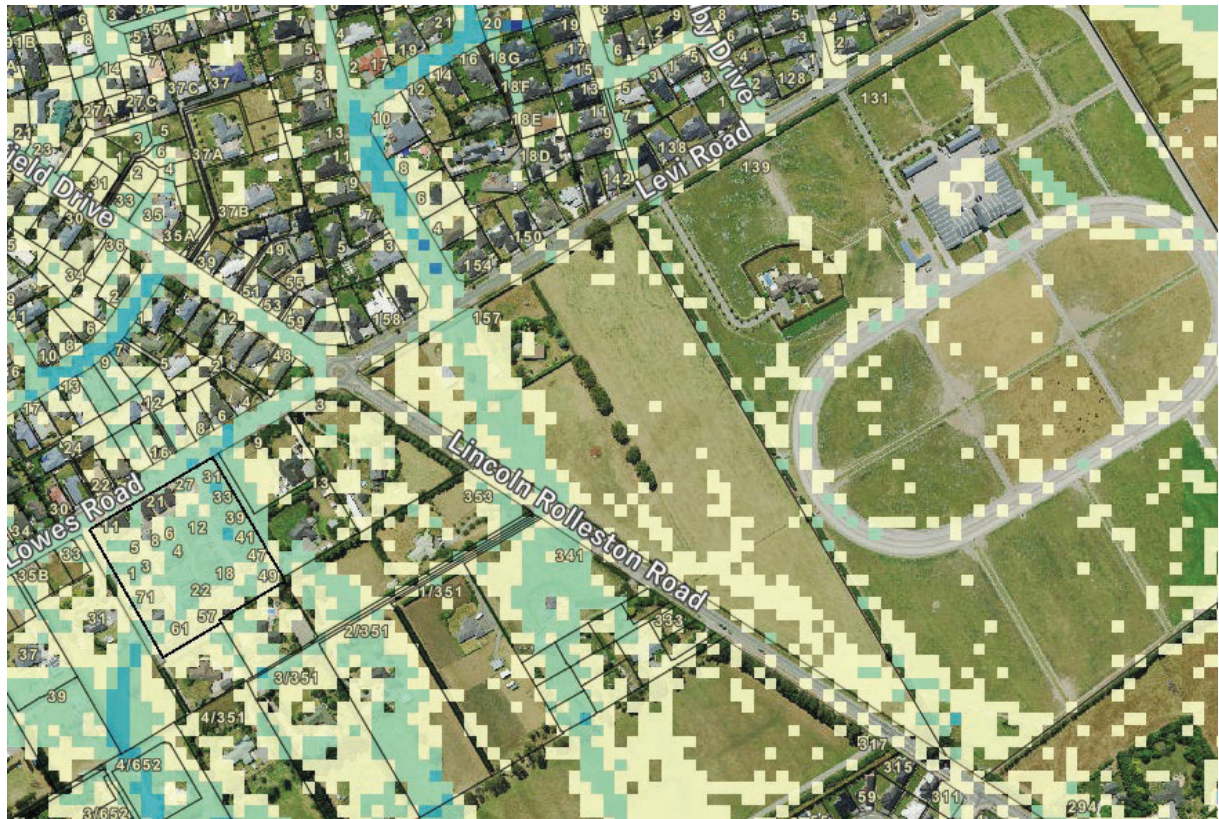
Figure 3 Flood Hazard Map for the 0.5% AEP (1:200 year) flood event
