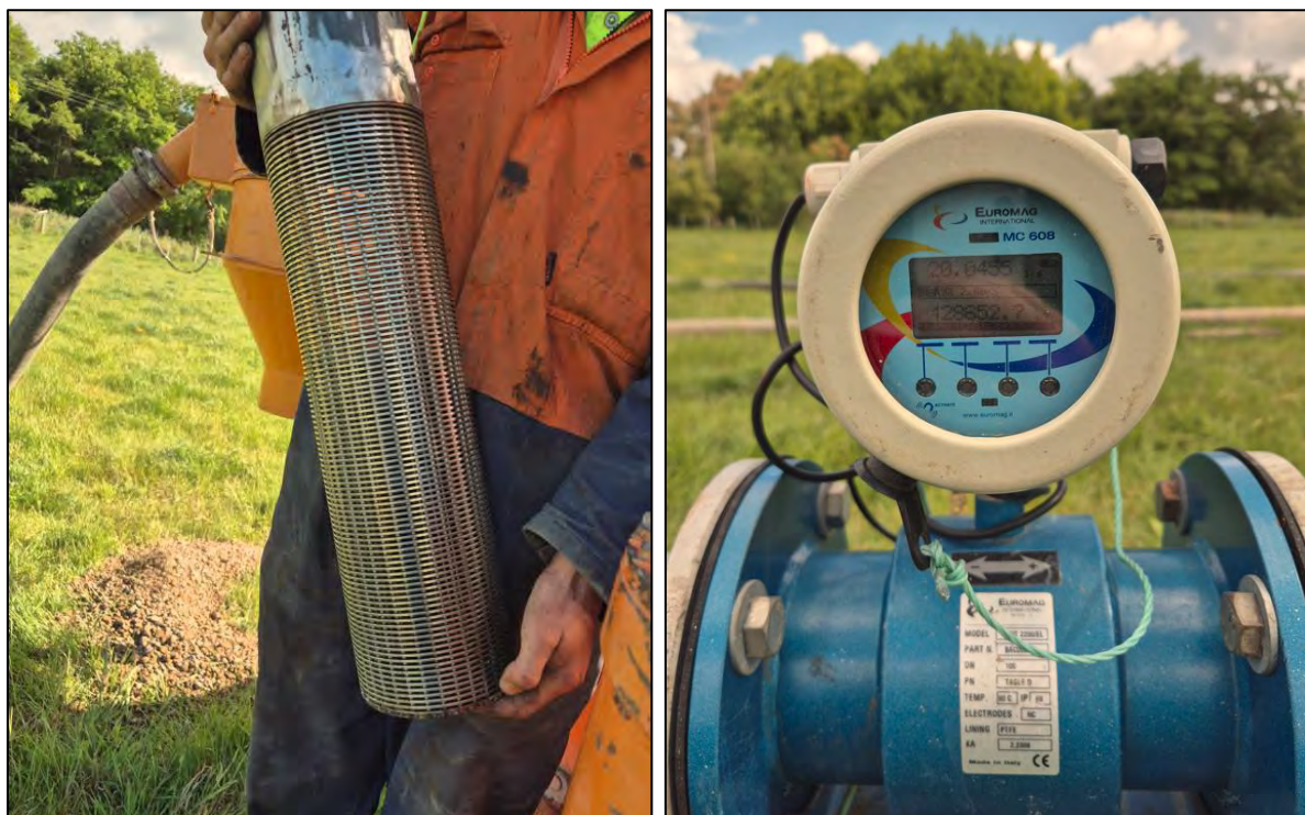
Figure 4: The 0.5 m long 3.5 mm gauge well screen inserted at the base of casing (left). Euromag flow meter with flow reported in litres per second and volume in cubic meters (m 3 ) providing values to the nearest to 0.1 m 3 increment.
