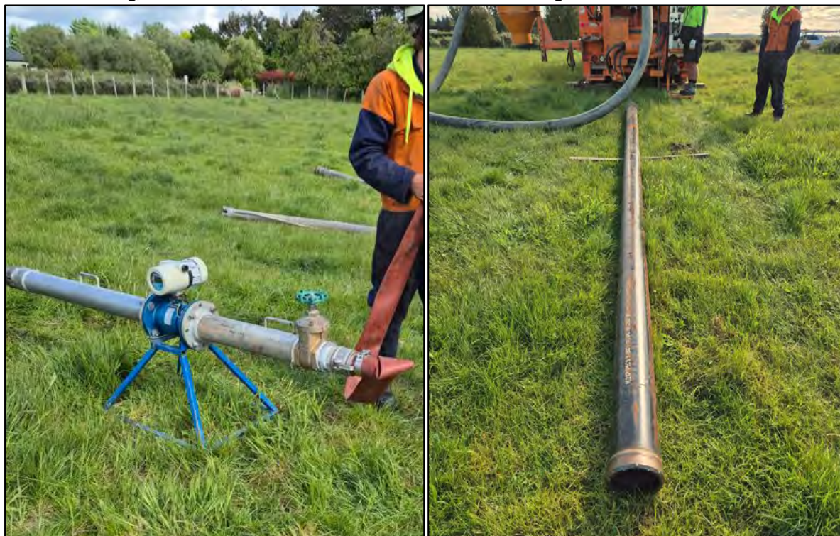
Figure 3: The flow meter used during testing set inline between water cart and top of steel casing (left). The 6 meter long, 154 mm ID, 184 mm OD steel casing prior to advancing into ground to 4.5m bgl for soakage testing.
