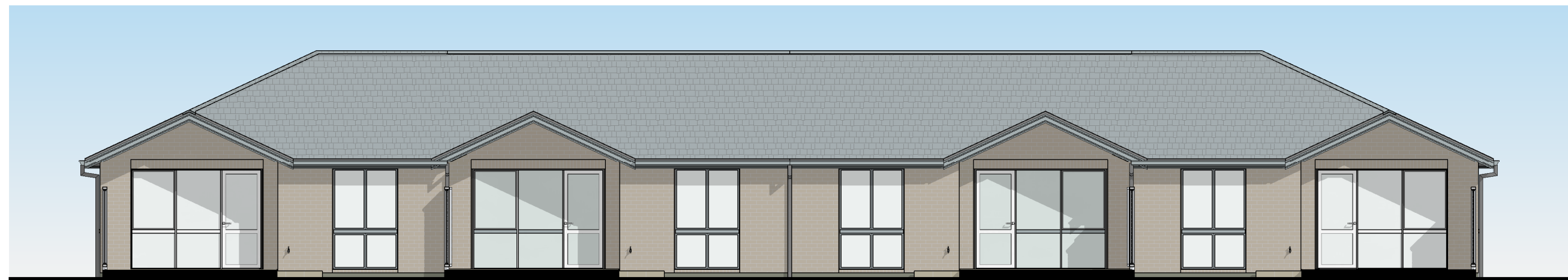
2 COTTAGE (NO GARAGES) 4 BLOCK - FRONT ELEVATION 1 : 100
