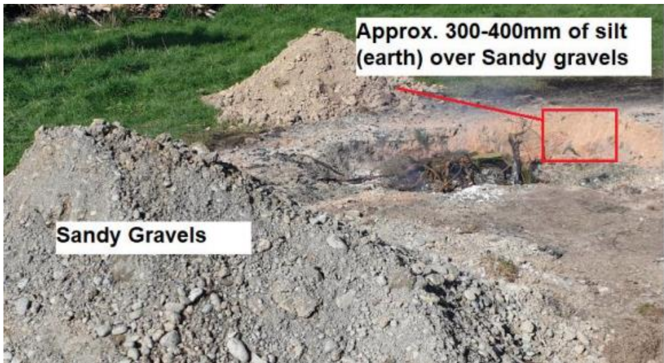
Figure 4 Excavated burn pit ground profile (source: Daniel Meehan)
