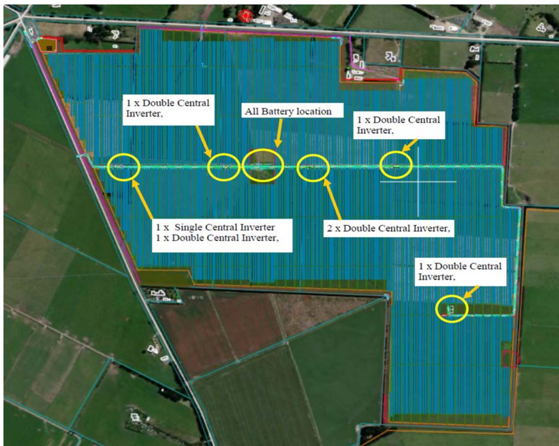
Figure 2: Site Layout and Battery Plan.
