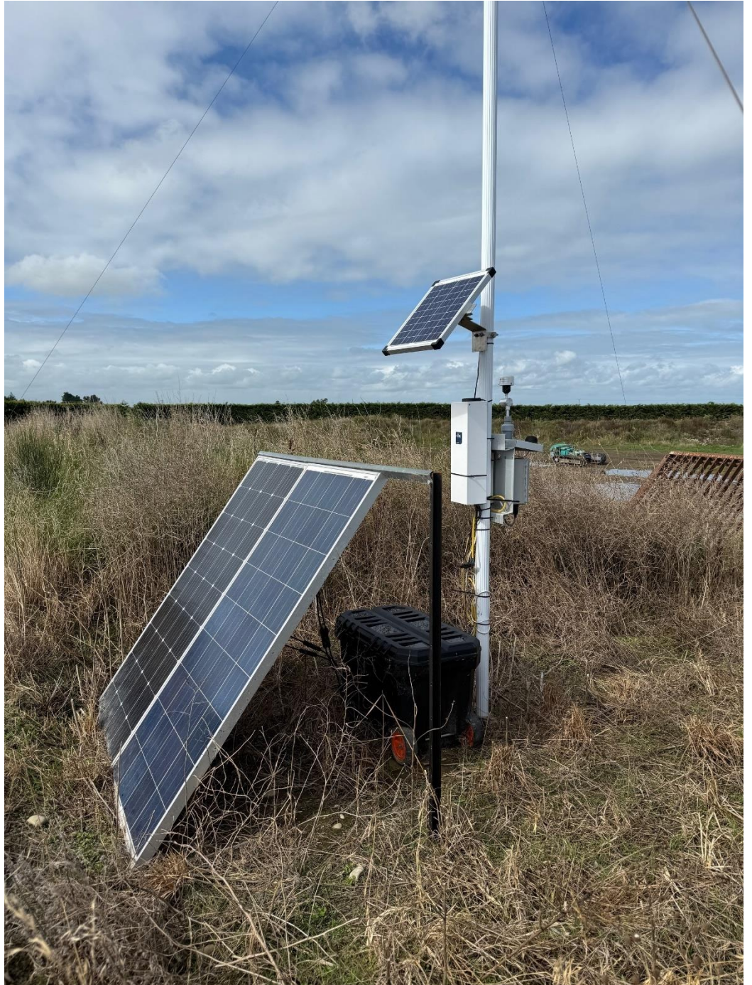
Figure 5. Photograph of the permanent dust and wind monitoring station mast
