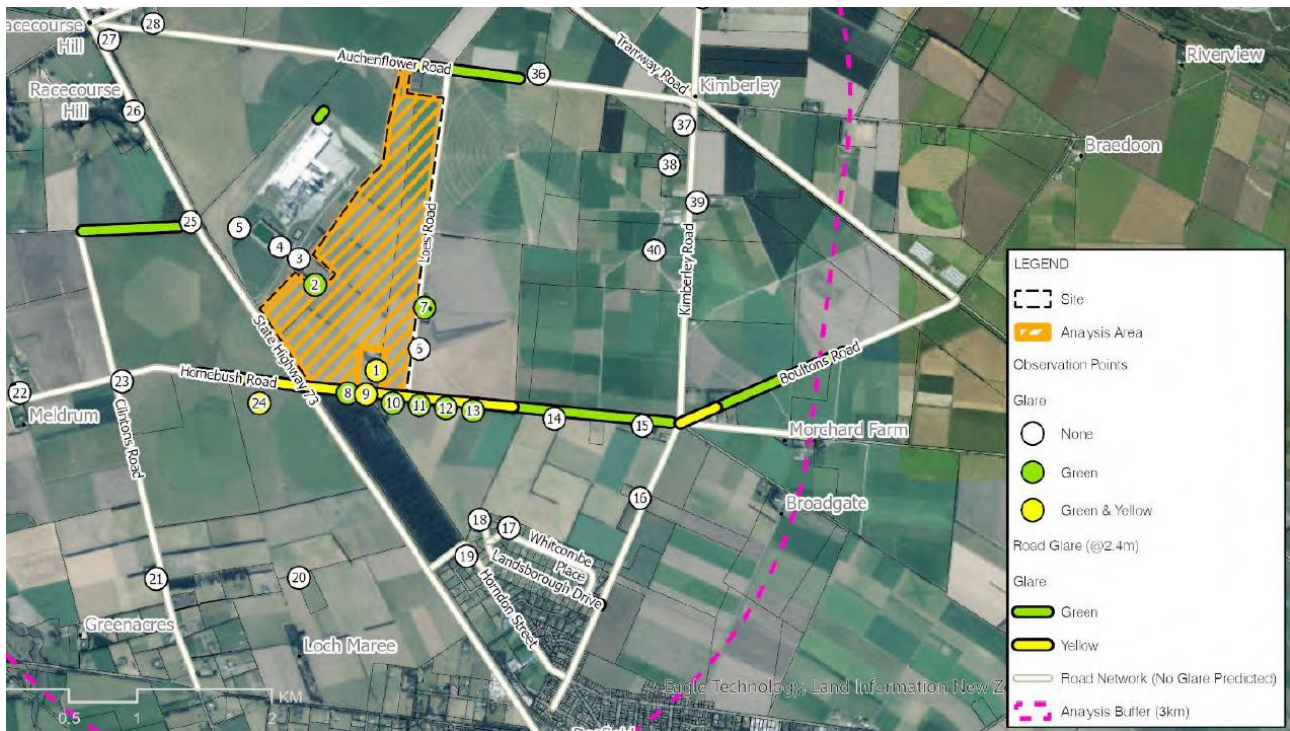
Figure 2.2 Locations where glint and glare are most likely to occur at different times of the day and year (reproduced from Glare Assessment)
