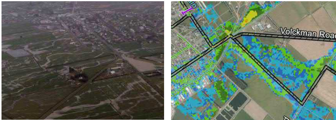
Figure 2 Comparison between Historic Flood Event Photograph and 1% AEP Design Scenario Flood Model Results.
