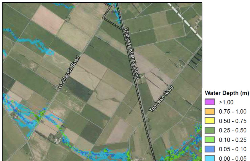
Figure 21: Existing Scenario - Peak Flood Depth and Inundation Extent at the Lake Road properties
