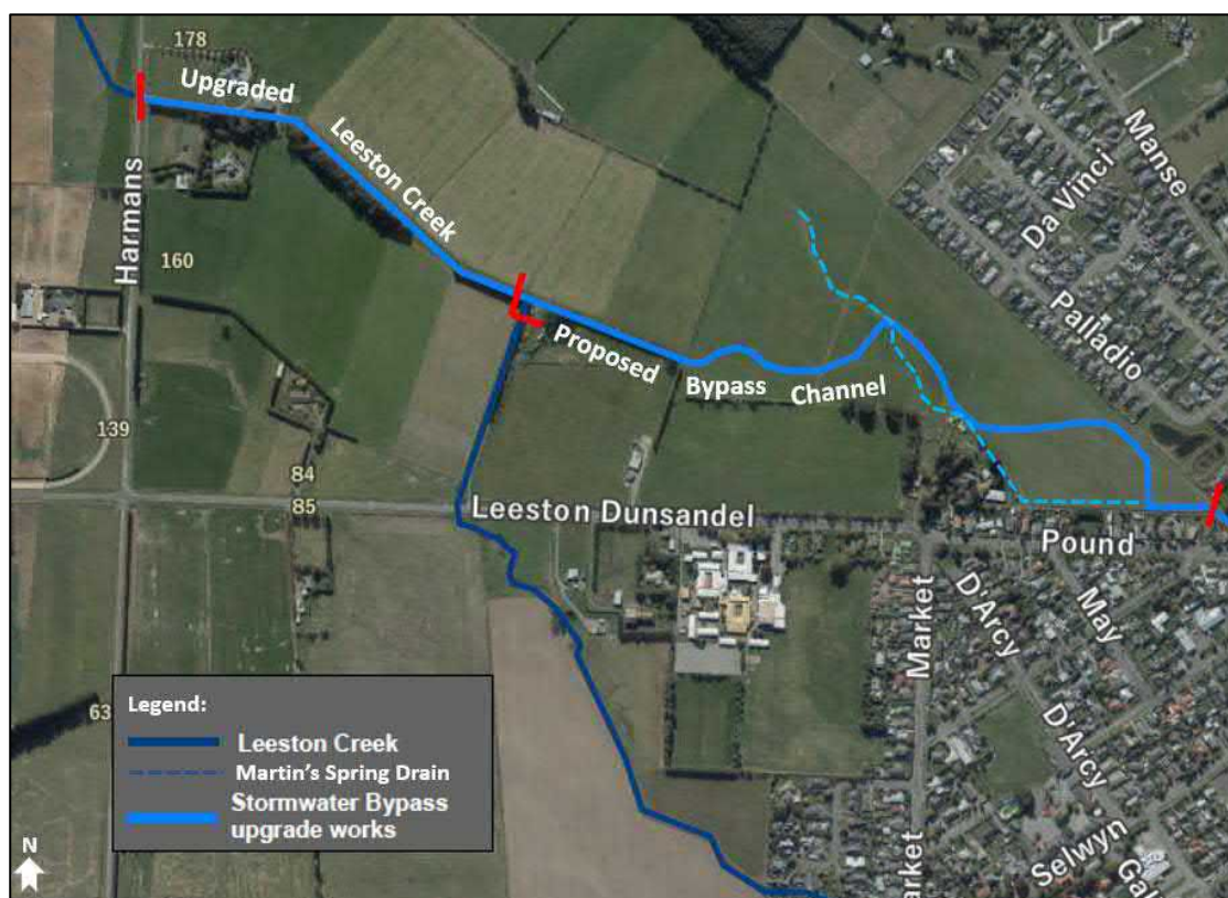
Figure 5: Proposed Bypass Channel and relationship to existing drainage network.
