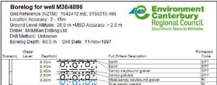
Figure 7 – Bore log M36/4896 is within 90m of the proposed twin culvert upgrade
