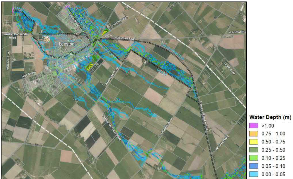
Figure 11: Existing Scenario - Peak Flood Depth and Inundation Extent.
