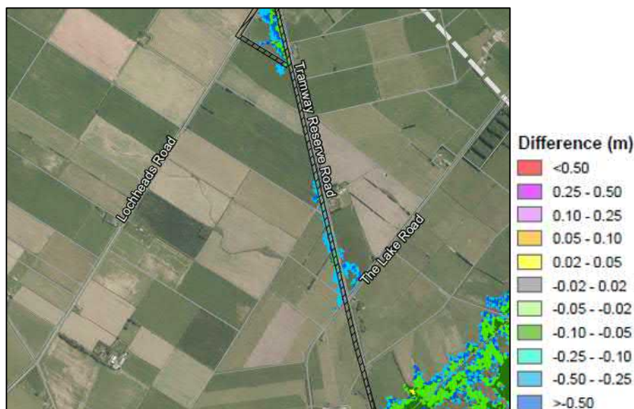
Figure 22: Changes in flood depth (pre-project vs post-project) at the Lake Road properties
