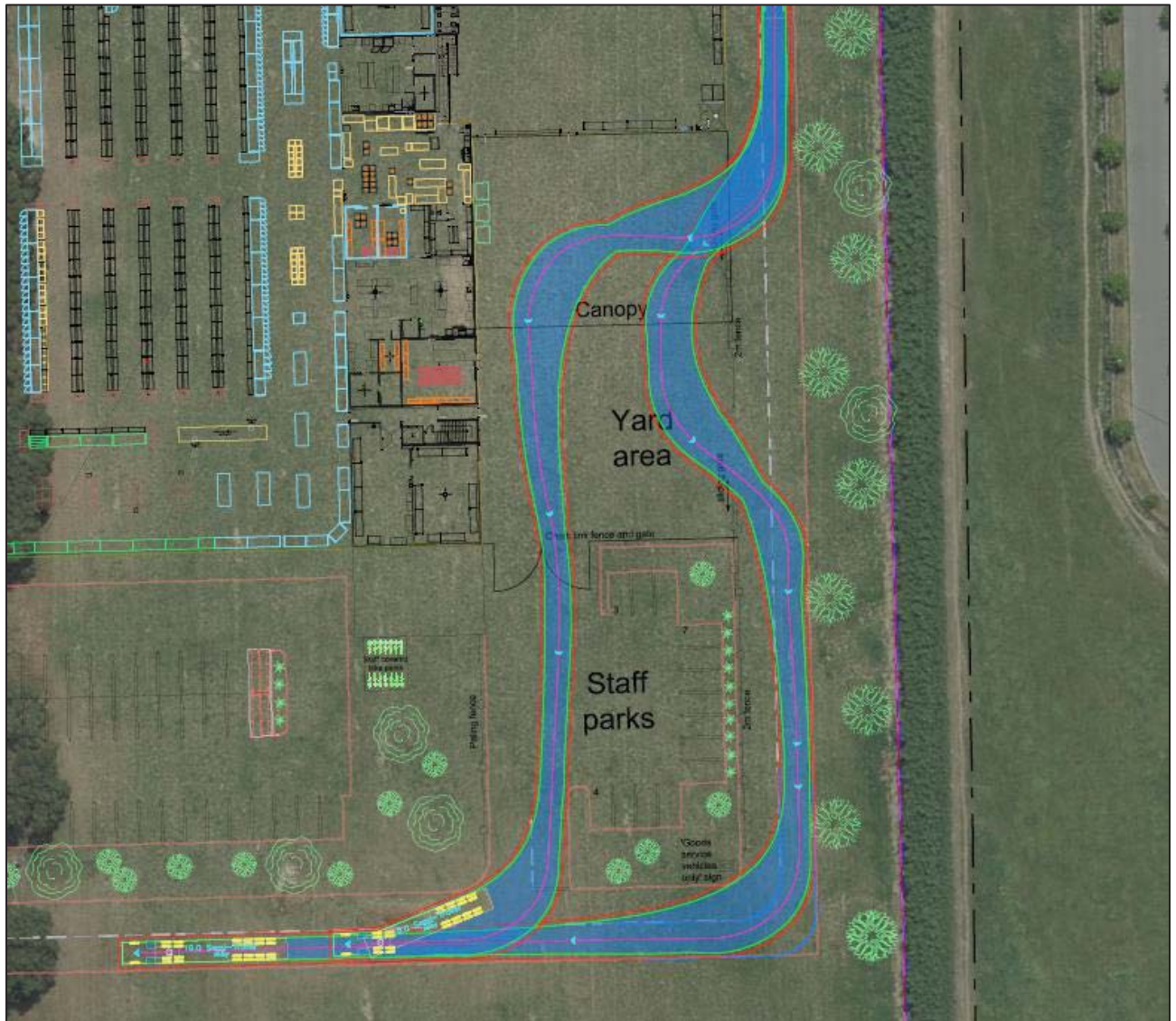
Figure 7.6 Vehicle tracking for a 19m semi-trailer truck within the yard area
