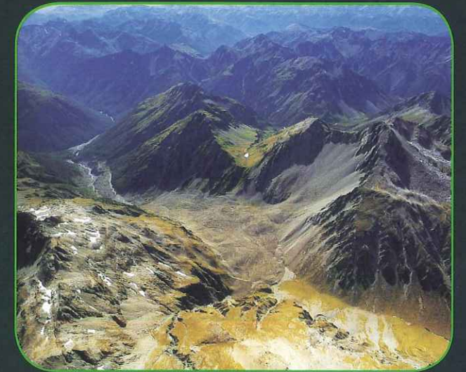
Above: Fifty-five million cubic metres of rock fell from Falling Mountain on the Main Divide during the 1929 Arthur's Pass earthquake and travelled 4.5km down the Oteha River.
