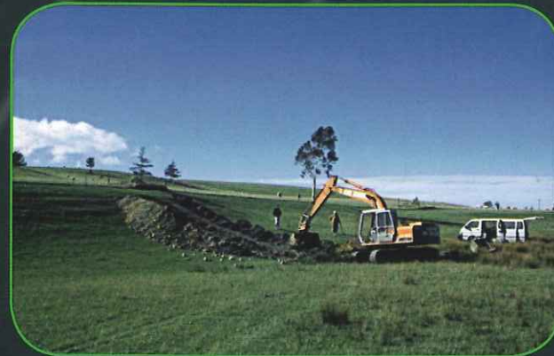
Above: Digging a trench across the Ashley Fault scarp near Rangiora. Trenching reveals where layers of sediment have been offset by movement on the fault during earthquakes. Organic material within the sediment can be dated to help determine when earthquakes have occurred.
