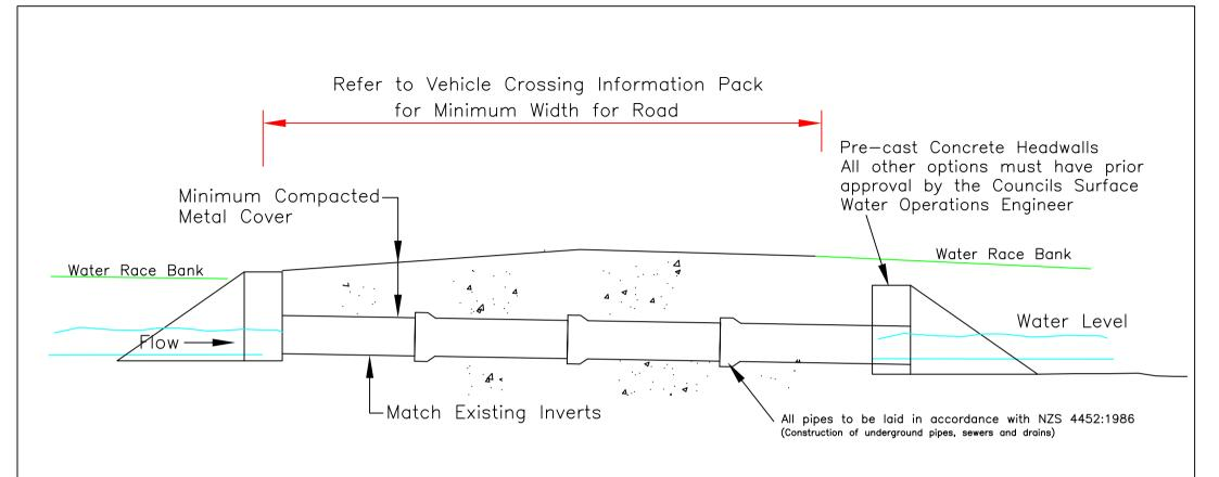
Culvert Size - Contact Councils Surface Water Operations Engineer for Culvert sizing Minimum Cover - Concrete class 4 pipes 600mm
