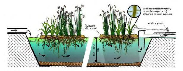
Figure 1. Cross section of FTW in a treatment pond (from Headley and Tanner 2011).
