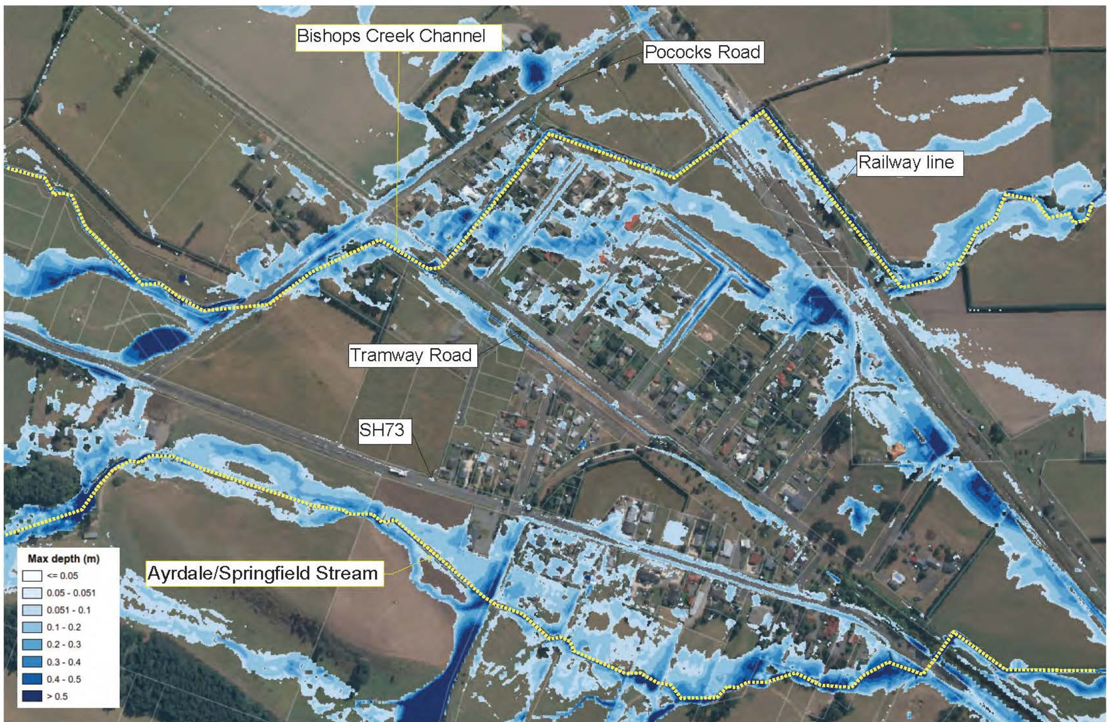
Flood map: 2% AEP flood event 6-hour duration with 20 m 3 /s diversion
