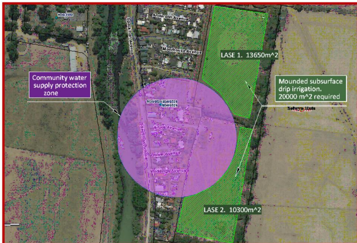
Figure A4. Option 2. 20,000m 2 raised irrigation field
