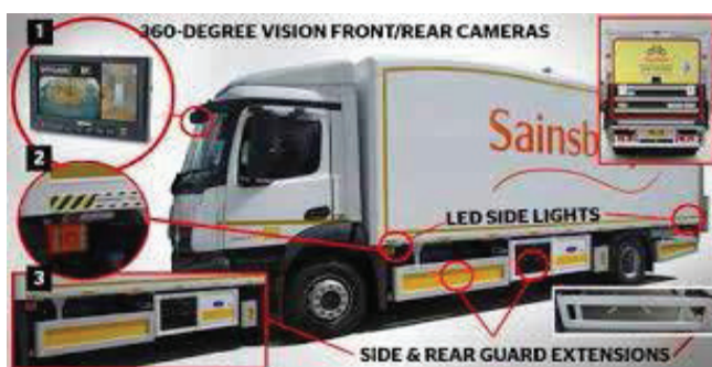
Graphic showing (1) the system of front, rear and side cameras; (2) new proximity sensors and LED indicators; (3) extended side and rear guards with reflective infills. (Source: Evening Standard)
