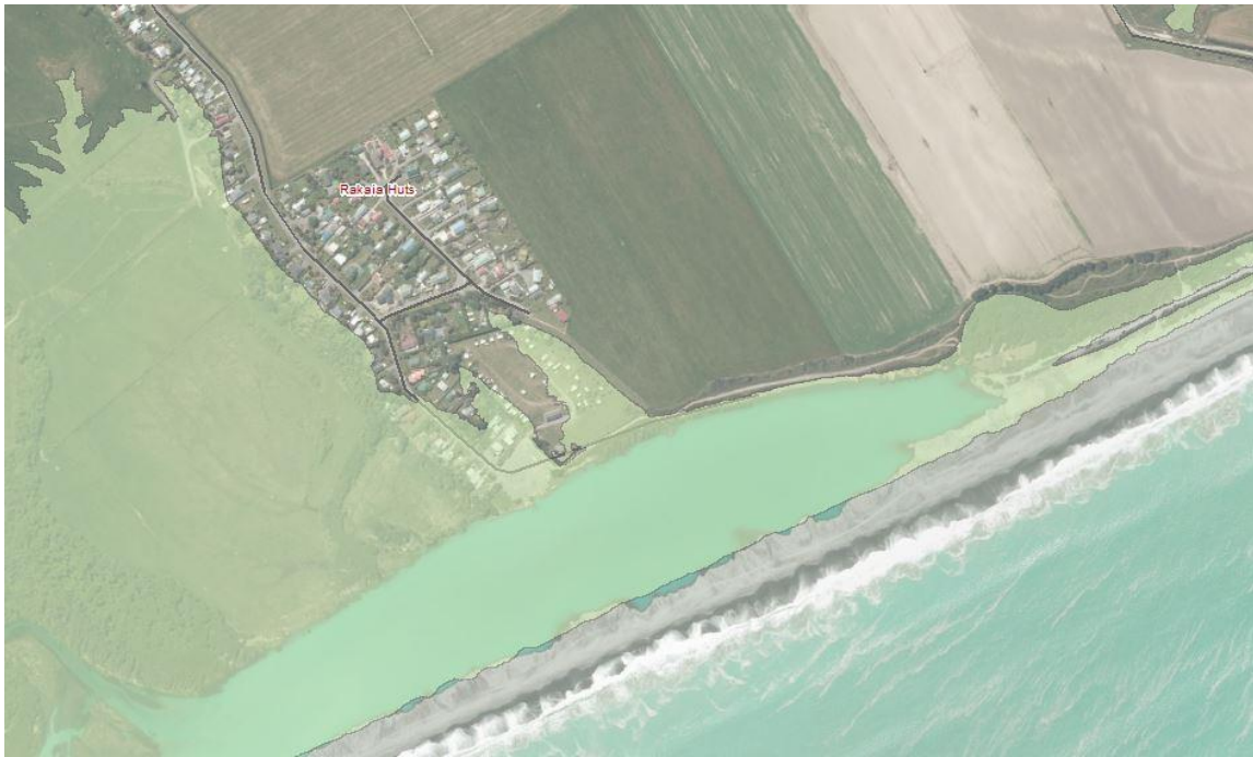
Figure 8-1: North Rakaia Huts and Rakaia River hāpua indicating land below 4 m elevation (above mean sea level LVD-1937)
