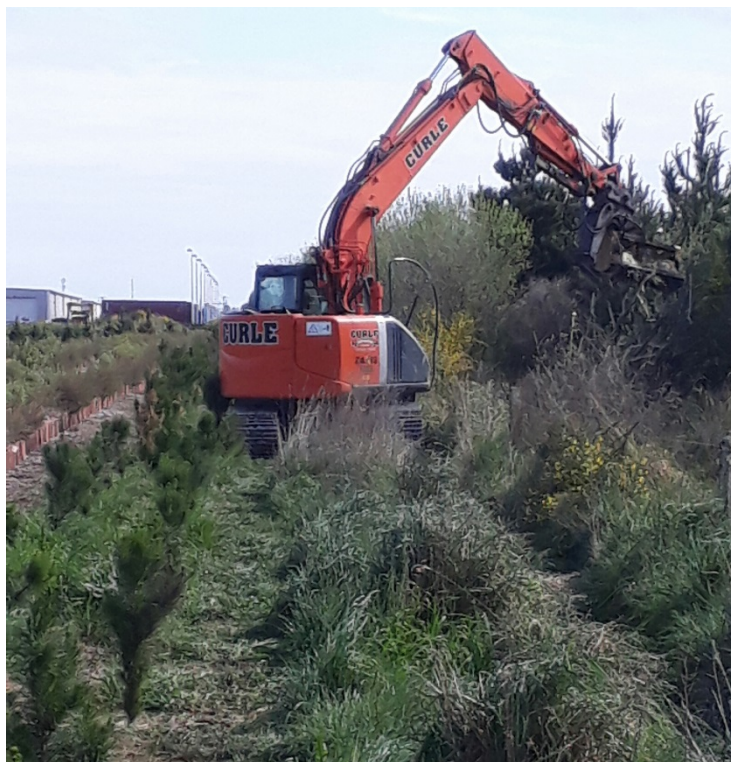
(Photo 3 – Mulching head on Digger – Note setback of planted trees)
